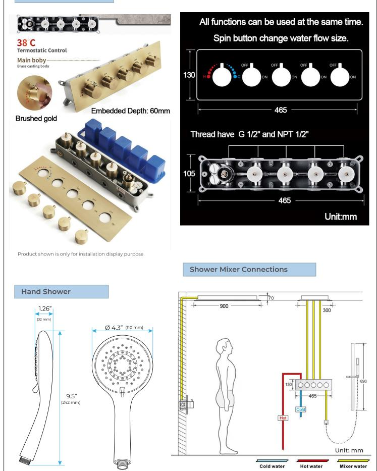
Flow Rate: 2.0 GPM / 7.6 LPM
